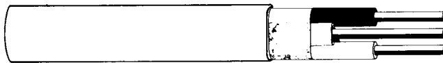
FIGURE 9.110 Type NM cable marked NM-B has insulation rated 90°C with a cable ampacity of 60°C.
