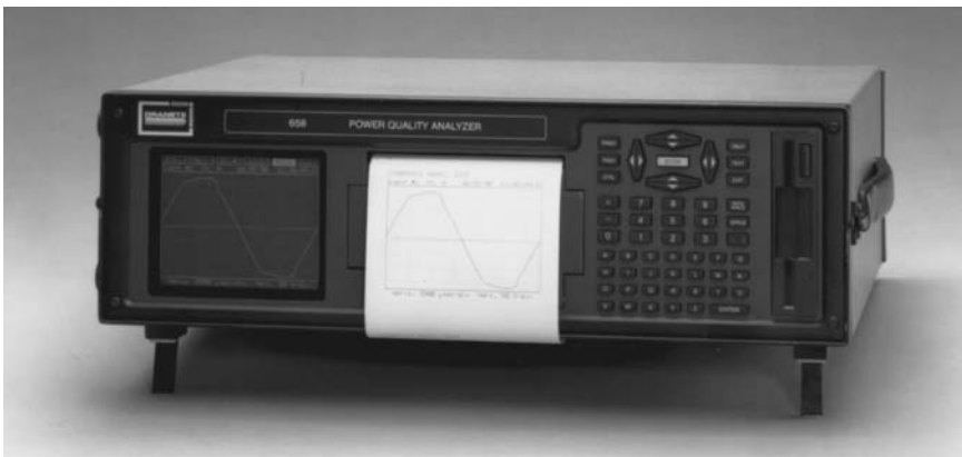
FIGURE 5.87 Analysis of power quality with a Model 658 digitizing oscilloscope, true RMS ammeter, true RMS voltmeter, harmonic distortion analyzer, power disturbance monitor, and strip chart recorder in one compact instrument. [Dranetz Technologies, Inc.]
