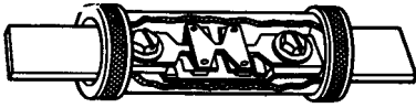
FIGURE 4.69 Cutaway view of time-lag fuse of the renewable type. [Superlag fuse of the Cooper Bussman, Inc.]
