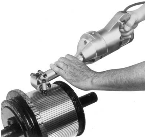
FIGURE 7.43 Hand-type mica miller. [The Martindale Electric Co.]
