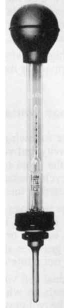
FIGURE 4.196 Vent-plug hydrometer syringe. [Electric Storage Battery Co.]
