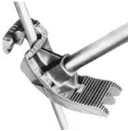
FIGURE 9.52D No. 9 Benfield double-grooved bender for 1/2-/3/4-in EMT and 1/2-in rigid conduit. Note that the handle has a weatherproof Zip Guide® plus an expanded end permitting its use as a stub straightener. [Jack Benfield, patent holder]
