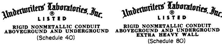
FIGURE 9.71 Identification of aboveground PVC conduits.
