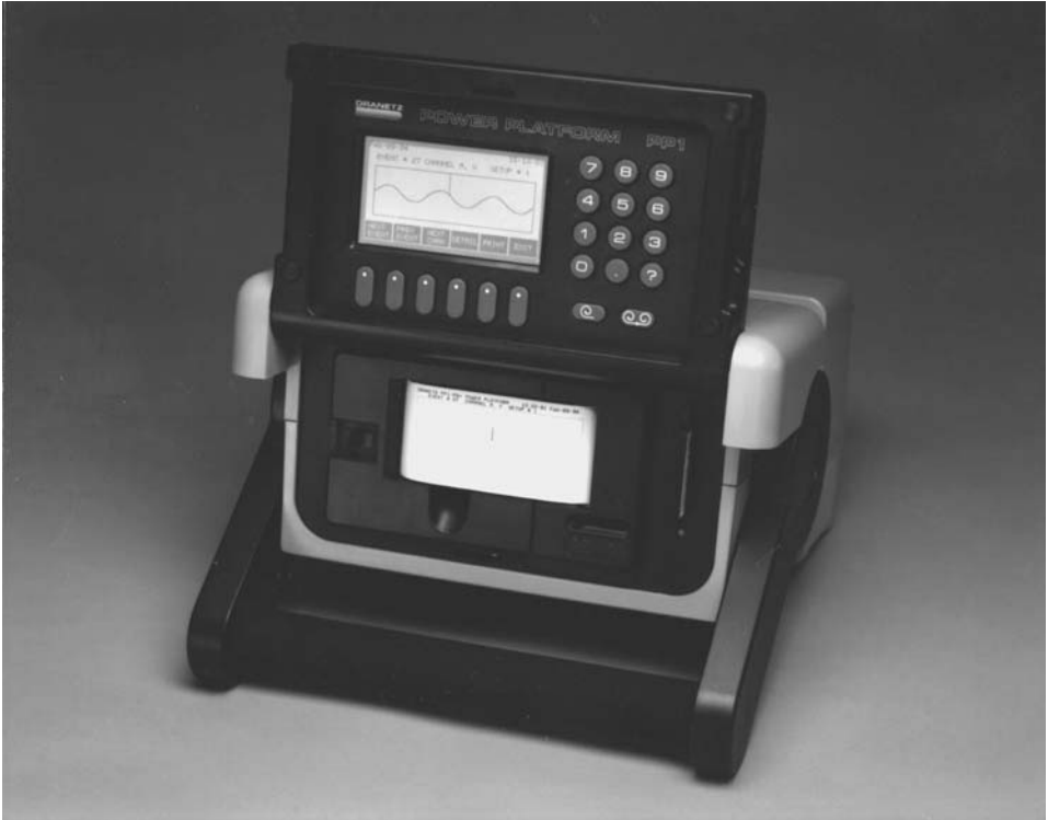
FIGURE 1.115 An 8-channel analyzer for capturing transients, voltage sags, swells, harmonics and other power disturbances. Used in conjunction with the PQ Task Card® the Power Platform® can generate reports and do K-factor computations for transformer selection. [Dranetz Technologies, Inc.]
