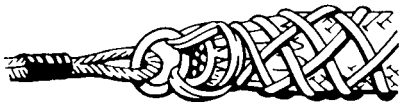
FIGURE 2.49 Use an insulated basket grip to attach a pull line to the conductors. A bare steel grip should not be used because it will score the inside of the conduit.
