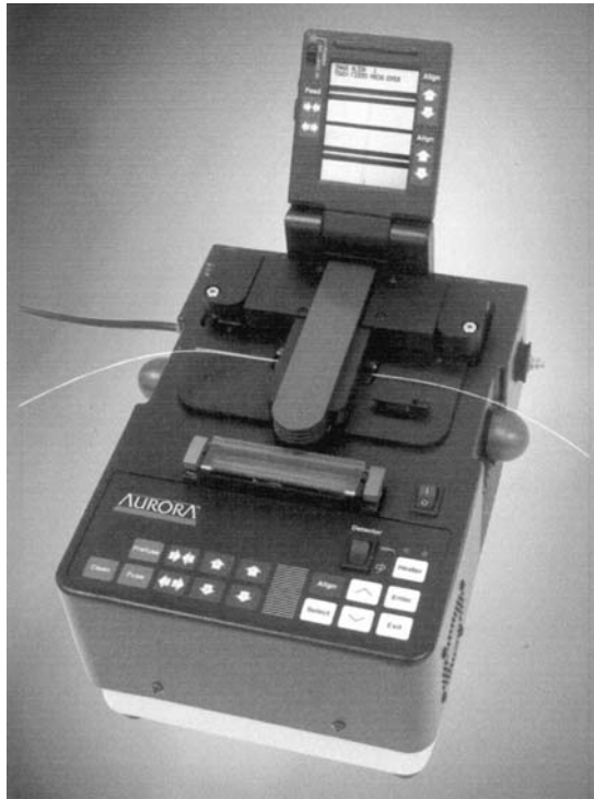
FIGURE 11.13 Fusion splicer. [Aurora.]
