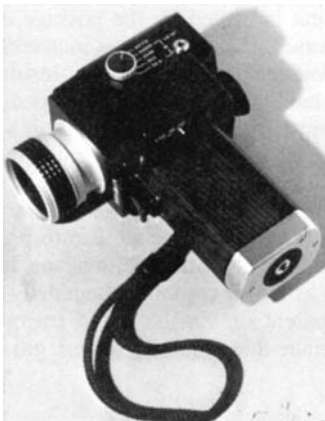
FIGURE 10.22 Portable brightness meter. [Minolta Corporation]
