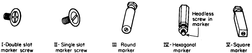
FIGURE 9.194 Markers for cellular-metal-floor raceways. [H. H. Robertson Co.]
