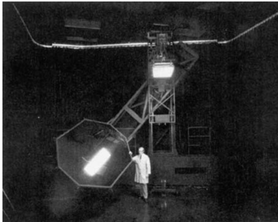
FIGURE 10.15 Mirror photometer used to measure the luminous intensity of a light source or luminaire in all directions. [General Electric Co.]
