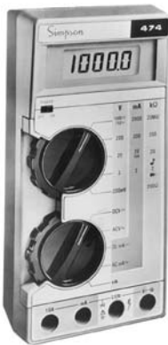
FIGURE 1.67A Hand-held digital multimeter. [Simpson Electric Co.]
