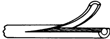
FIGURE 2.44 Another safe method of removing insulation from conductors is to peel the insulation back and then cut outward.
