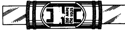
FIGURE 4.68 Knife-blade-contact time-delay renewable cartridge fuse. [Reliance Fuse Division of Reliance Electric Corp.]
