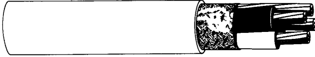
FIGURE 9.126 Four-conductor Type SE cables uses three insulated conductors and a bare equipment ground.
